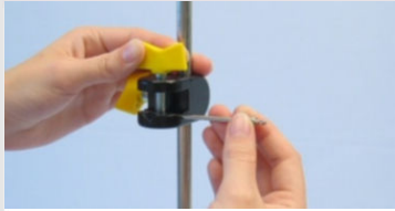
Fix holding pin at bosshead
